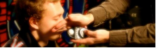
The device that determines exposure is called a light meter.
