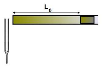
In the second trial, the students use a tube with a constant length, but they place in the tube a cork stopper with the same diameter as the inner size of the tube. The cork cn freely move from the left side of the tube to the right. The frequency of the tuning fork stays the same as it was determined in the first trial.
