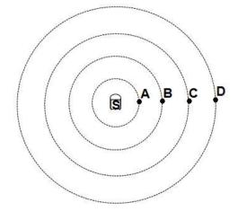
3. A sound source S radiates a sound wave in all directions. The relationship between the distances is SA = AB = BC = CD. Which of the following points oscillates at the highest frequency?
