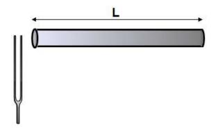
4. A group of students in a physics lab perform a series of experiments with a set of tubes and tuning forks. In the first trial, they use a tube whose length can be extended. The length of the tube when sound resonates for the first time is 1.0 m. ( $v_{sound} = 340 \text{ m/s}$ )
