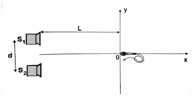
3. Two loudspeakers separated by a distance d = 0.75 m are placed at a distance L = 4 m from the y-axis. The loudspeakers generate waves with the same frequency f = 680 Hz and amplitude A. The waves oscillate in phase. When a microphone moves in parallel to the y-axis, it can detect points with no sound or sound of maximum amplitude. (V<sub>sound</sub> = 340 m/s)
