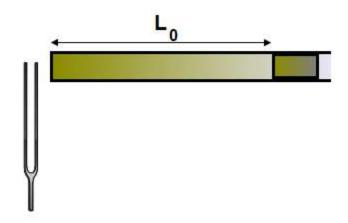
In the second trial the students use a tube with a constant length but they place in the tube a cork stopper with the same diameter as the inner size of the tube. The cork can freely move from the left side of the tube to the right. The frequency of the tuning fork stays the same as it was determine in the first trial.
