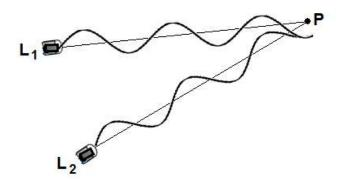
25. Two loudspeakers generate sound waves with frequencies of 680 Hz. What is the extra distance traveled by the second wave if a stationary observer detects maximum intensity of sound at point P?
