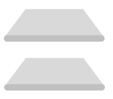
When a battery is connected to the plates, charge moves between them. Every electron that moves to the negative plate leaves a positive ion behind.
