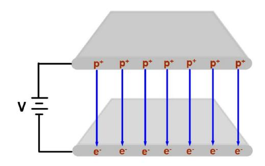
Drawing the Electric Field from the positive to negative charges indicates that the Electric Field is uniform everywhere in a capacitor's gap.
