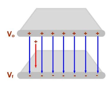
24 The positive charge moves from the top plate to the bottom plate, at a constant velocity, in the below configuration. What is the work done by the Electric Field on the charge?
