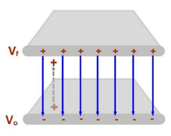
28 If a positive charge moves upwards in the following diagram with a constant velocity, what is the work done on the charge by the Electric Field?
