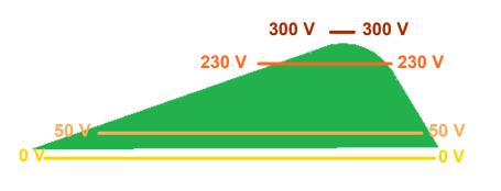
These "topography" lines are called "Equipotential Lines" when we use them to represent the Electric Potential - they represent lines where the Electric Potential is the same.
