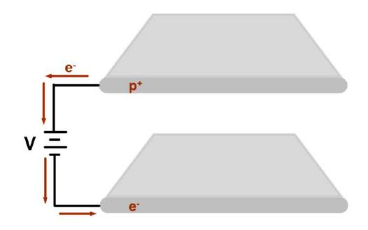
The electrons are attracted by the positive terminal of the battery and move through the wire and the battery to arrive on the other plate.
