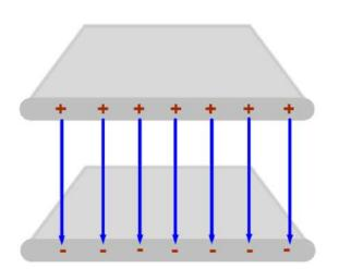
Let's begin by examining two infinite planes of charge that are separated by a small distance.
