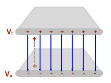
29 If a positive charge moves upwards in the following diagram with a constant velocity, what is the work done on the charge by the external force?
