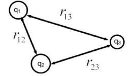
5 Compute the potential energy of the three charges in the following configuration:
