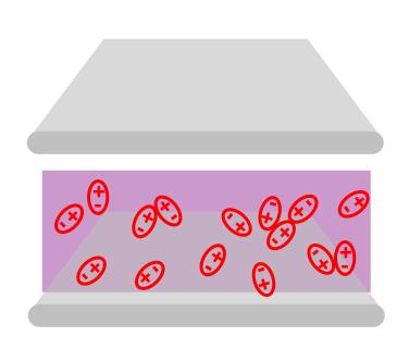
When the plates are charged, the atoms line up with their negative ends closer to the positive plate - the dielectric material is polarized.
