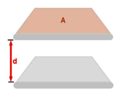
45 A parallel plate capacitor has a capacitance C<sub>0</sub>. If the area on each plate is doubled and the distance between the plates is cut in half, what will be the new capacitance?
