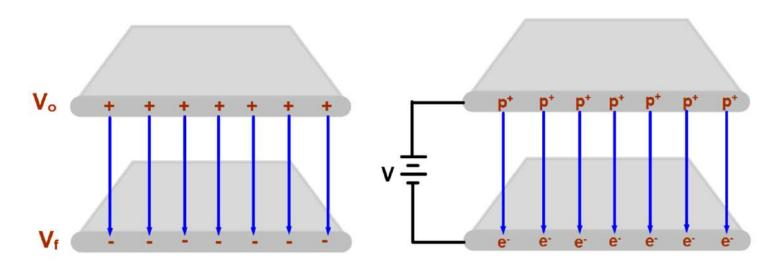
The parallel plates of the capacitor have a finite size, but they are designed so that the plate size is very much greater than the distance between them - so the capacitor properties are very close to the infinite plane case.
