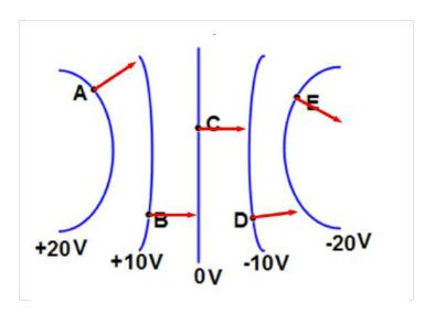
This configuration is created by a positive charge to the left of the +20 V line and a negative charge to the right of the -20 V line.
