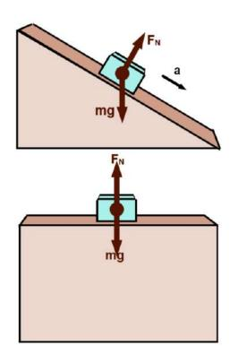
Consider a mass on an inclined plane. The slope of the plane determines the acceleration and the net force on the object.
