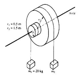
3) Two masses.  $m_1$  and  $m_2$ , are connected by light cables to the perimeters of two cylinders of radii  $r_1$  and  $r_2$ , respectively, as shown in the diagram above with  $r_1 = 0.5$  meter,  $r_2 = 1.5$  meters, and  $m_1 = 20$  kilograms. a. Determine  $m_2$  such that the system will remain in equilibrium.
