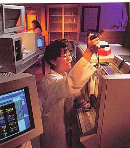
This scientist is using an automatic pipette to deliver a fixed volume of liquid into a sample cell.
