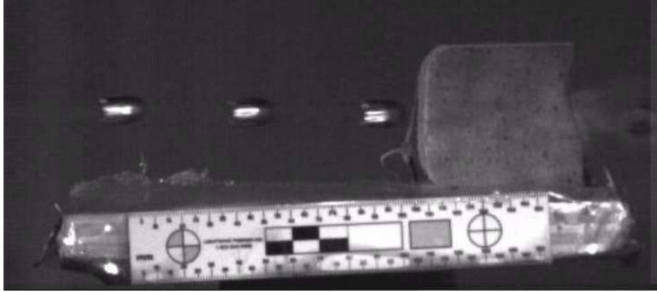
Figure 2: Superimposed time lapse images of a single .45 caliber bullet impacting a blood-soaked sponge, recorded at 10,000 frames per second. The first three bullet images are separated by 0.2 ms; the spatter at far right occurred 0.4 ms later. The black rectangles on the scale bar are 1 cm in length.
