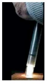
In the video you see a syringe and a piston that snugly fits into it. At the end of the piston is a small hook to which a small piece of cotton ball is tied. The experimenter is holding the syringe vertically and suddenly presses down hard on the piston. The high-speed video (recorded at 1200 frames per second) shows what happens:
