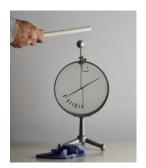
**a.** Charge a foam tube with any material and then bring it close to the top of the electroscope without touching. Observe what happens when you are holding the tube close and explain your observations. Then remove the tube, observe what happens and explain.
