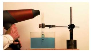
The goal of this activity is to determine the same physical quantity using two different methods. The physical quantity is the speed of the air exiting a hairdryer. You can either repeat the experiments, described below, yourself and collect similar data or you can use the data provided below. After you determine the speed using two methods, compare the results. Are they the same or different? How certain are you in each of the values?
