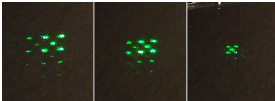
Fig. 5. Experimental patterns observed on the surface of mirrors with progressively decreasing thicknesses (from left to right). The distance between the camera and the mirrors and settings of the camera were the same in all cases.
