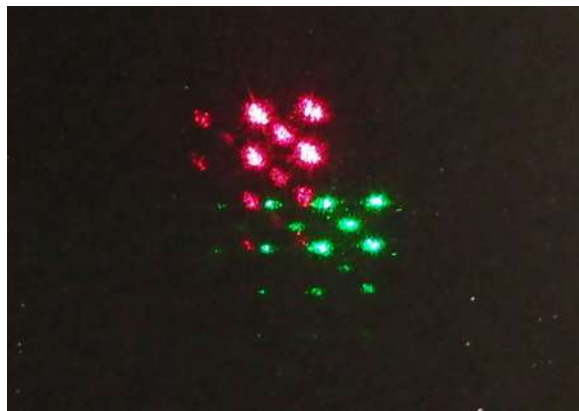
Fig. 4. Observed pattern for red and green lasers simultaneously shining on the mirror. (Color online)
