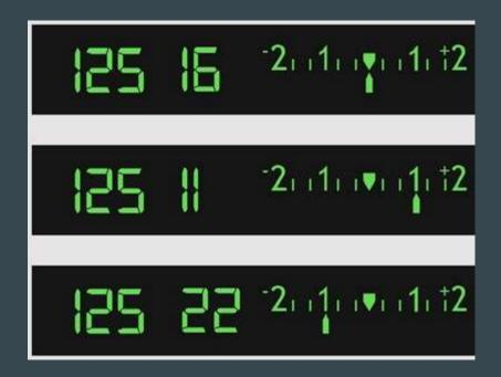
In these examples, the shutter (1/125) stays the same, and the aperture is changing. By looking at the light meter, we can see that the amount of light let in has changed.
