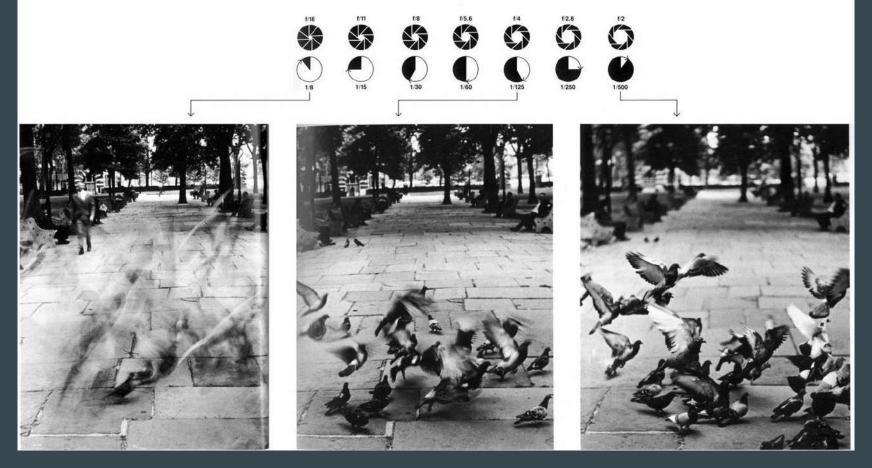
We already know that shutter and aperture are the 2 ways to let in light into the camera. We also know that the visual effect of the shutter speed is how motion is shown, and that aperture controls the depth of field.
