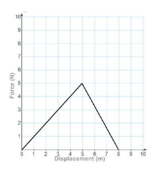
13. The force as a function of displacement of a moving object is presented by the graph. How much work is done when the object moves from 5 m to 8 m?
