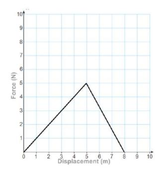
12. The force as a function of displacement of a moving object is presented by the graph. How much work is done when the object moves from 0 m to 5 m?
