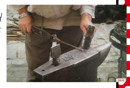
After quickly removing the red-hot piece of iron from the fire, he placed it on the anvil, and started to bang away at it with his hammer. In this picture you can see the anvil--the big block of metal on which the blacksmith shaped the iron.
