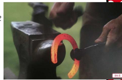
When he was happy with the size and shape of whatever he was making, the blacksmith would let the iron cool off, sometimes by plunging it into a bucket of cold water, and it would harden. What would make the iron harden faster, leaving it out in the air or plunging it into the cold water? Why?
