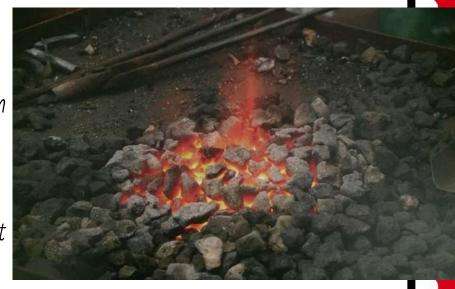
Once the forge was hot enough, the blacksmith would put a piece of iron in it. Because the forge was so hot, he had to use tongs. Tongs have two long metal arms connected by a hinge.
