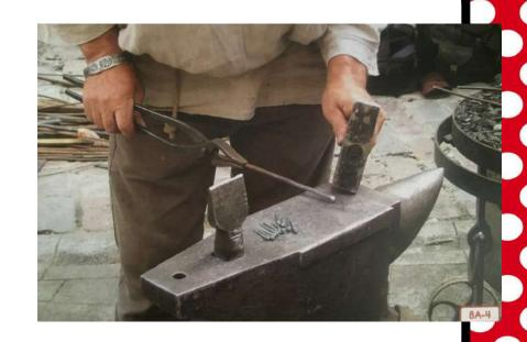
As long as the blacksmith kept the metal hot, he could shape it however he liked. He could make the metal longer or shorter, thicker or thinner. He could bend it and mold it into special shapes. In this picture you can see how the blacksmith ĭs shaping a horseshoe.
