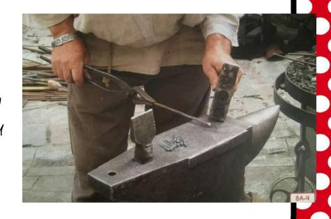
The blacksmith had to work quickly, because the metal was only soft and pliable when it was red hot. Once the iron cooled, it would harden.
