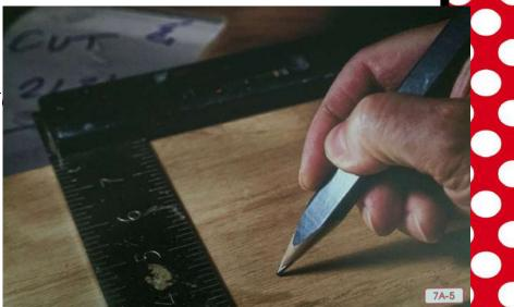
Most good carpenters measure their boards twice before cutting, just to make sure that they have marked the exact, right place. That's why carpenters have a saying: "Measure twice; cut once." It's basically to remind themselves to double check their measurements before cutting. Once they cut a board, they can't uncut it.
