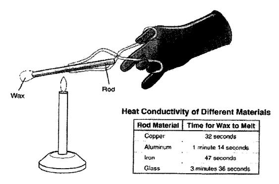
Which list shows the correct order of the substances from the most to least efficient at conducting heat?
