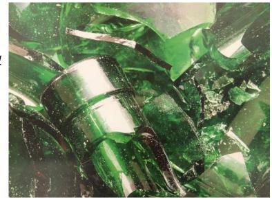
Here is a little piece of glass that has has been heated up so much that it is just about to melt and turn to liquid. Now imagine a big pot full of little bits of glass like this, all eventually melting together into a thick, hot, syrupy liquid. That's what you would find at a glass recycling factory.
