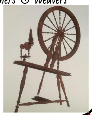
The spinning wheel not only has a spindle attached to it, but it also has a big wheel and a foot pedal called a treadle. The spinner would step on the treadle to make the big wheel spin; this was called treadling.
