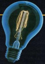
▲ TUNGSTEN Although tungsten can be combined with steel to form a very durable metal, in its pure form it is soft enough to be stretched to form the filament of a lightbulb. Tungsten has the highest melting point of any metal.
