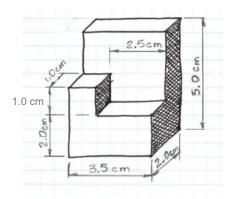
10. Create a **full scale isometric** view of the object represented in the following sketch using the dimensions shown. Use a metric ruler to obtain the correct dimensions on your sketch (If the height of the drawing in #9 is 5 cm then the isometric drawing needs to be 5 cm as well).
