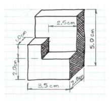
Cavalier Oblique. The sketch is an oblique pictorial since the front view is drawn "straight on" Depth of 2.0cm is the same measurement as the height of 2.0cm so it must be full depth. If the depth of 2.0 cm was half of the height of 2cm it would have been cabinet but it is not the came
