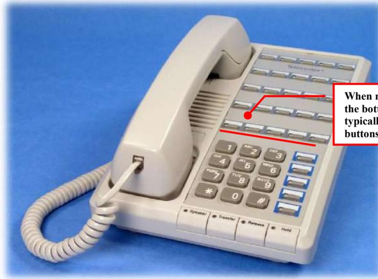
When multiple extensions are present, the bottom line of feature buttons are typically programmed as extension buttons.
