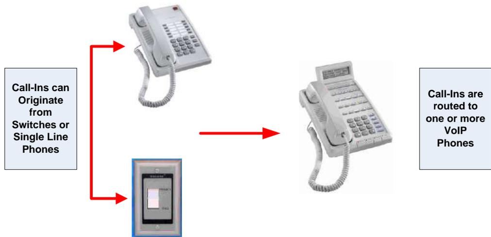
Figure 24: Call-in Routing 1 (Switch or Single Line Phone to VoIP Phone)
