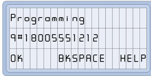
Figure 43: SD/DSS Button, External Number (with Programmed Pause After Access Code)
