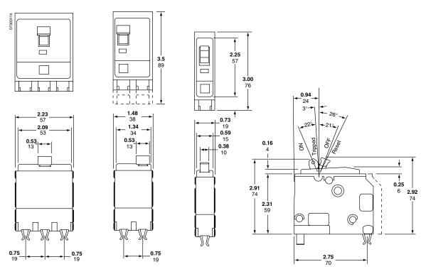
Figure 11: Type QOB Bolt-On Circuit Breaker
