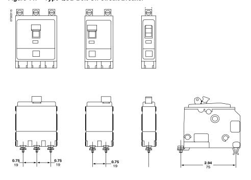
Figure 12: Type QO-GFI Circuit Breaker
