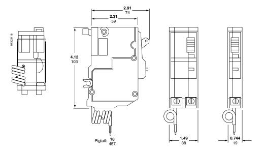
Figure 13: Type QO-AFI and QO-AFCI Circuit Breakers
