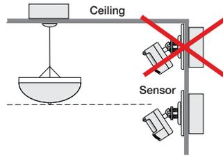
Mount LMPX-100-3 and LMPX-100-4 sensors at least 15' and not more than 30' above the floor. To suspend the sensor from a fixture or solid construction material, use the MB-1 Sensor Bracket.
