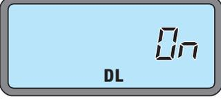
Once a parameter value is modified, a quick press on the "Feature" button displays the next available parameter. (DL is DayLighting.)
