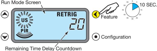
Press and hold the “Feature” button for 10 seconds. The LCD display shows “CLr” to confirm the sensor has been reset.
