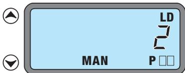
A quick press on the Configuration button steps through the loads connected to the DLM Local Network. The LCD display shows the selected load "LD #" and its associated parameters. At this point, one load is ON, and all switch buttons and sensors that are bound to this load have their blue LED solid ON.
