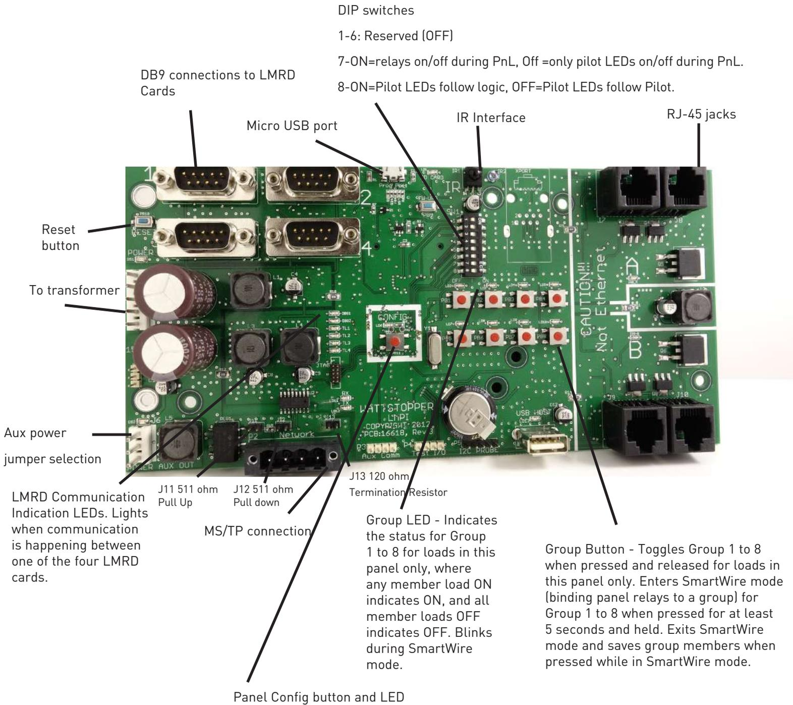
Figure 11: LMPI Circuit Board
