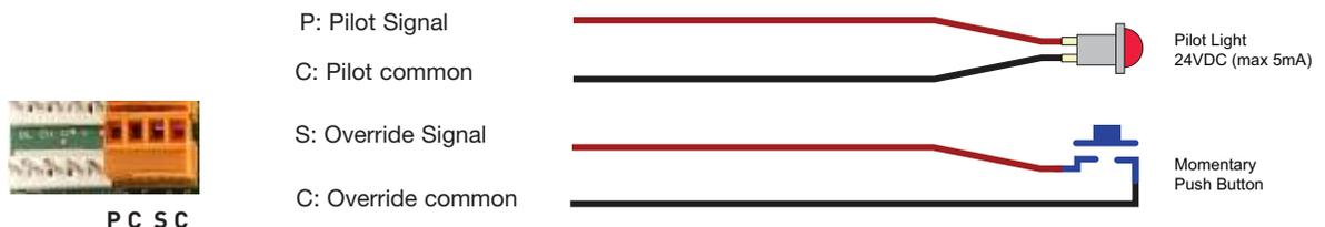
Figure 9: 2-wire momentary switch wiring
