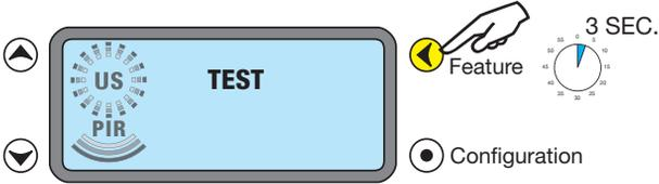
minute period is over, the sensor begins operating with the selected time delay. **To activate the test mode:** While TEST is in the sensor display, press and hold the Feature button for 3 seconds.
