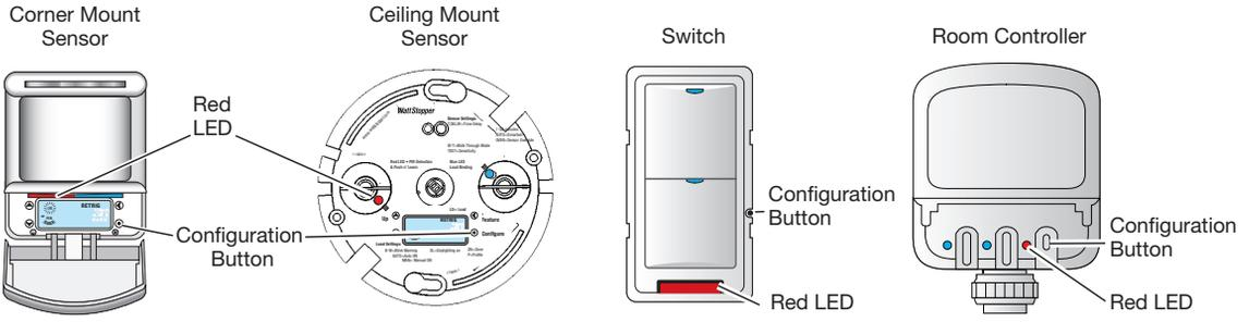
To enter PnL press and hold the Configuration Button on any DLM device. Release the button when the device's Red LED begins blinking (about 3 seconds).
