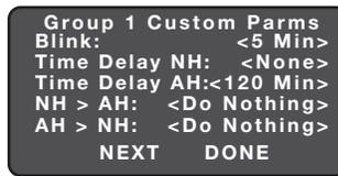
Specify a Blink Warning Interval of None (no blink) to 120 minutes. A time delay of 0 to 120 minutes can be specified for operation during Normal Hours and After Hours. What is supposed to happen to the group on a transition from Normal Hours to After Hours, as well as After Hours to Normal Hours is also specified (Do Nothing, Turn On, Turn Off. Pressing DONE will return to the Group Setup Menu.
