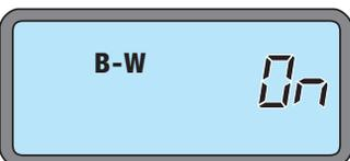
**Blink Warning (B-W):** When enabled "B-W" shows in the display. This function can be either enabled or disabled. When 1 minute is left on the time delay, the load controlled by the sensor turns OFF for 1 second then turns back on. This provides a visual warning before the load(s) are turned OFF by the sensor. By default Blink Warning is disabled (OFF).
