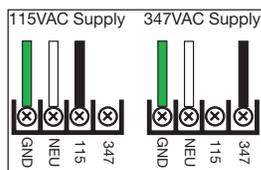
Figure 5: P115/347 wiring
