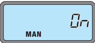
**Manual-ON:** in this mode, a DLM switch is required to turn ON the load. The sensor is then used to keep the load ON, based on occupancy activity. After the time delays elapses, the switch must be used to turn the load ON, if no movement is detected within the 10 second retrigger period.
