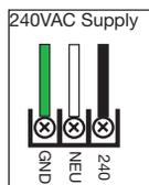
Figure 6: P240 wiring
