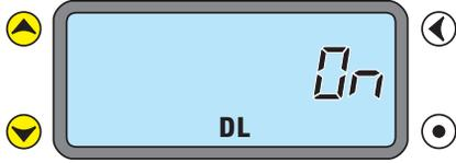
◀ **Daylighting (DL):** When this function is enabled “DL” displays. This function allows specific load(s) to be bound to a DLM daylight sensor, LMLS-10x series. By default Daylighting is enabled for load 1 and disabled for all other loads.
