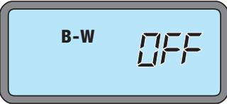
Once a load is selected, use the "Feature" button to cycle through the load parameters. (B-W is Blink Warning.)
