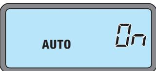
**Auto-ON:** in this mode, either a DLM occupancy sensor or switch can turn ON the load. A switch provides the following additional functionality:
