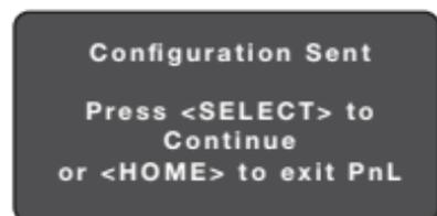
New settings have been sent to the selected load. Wait 5-6 seconds for the message to clear. Select another function (bind, next, exit). To instantly end load configuration press the HOME key.
