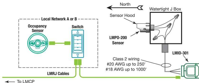
Figure 8: Connection of LMCP to LMIO-301
