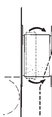
4. Unfold rubber collar over the reel's socket.
