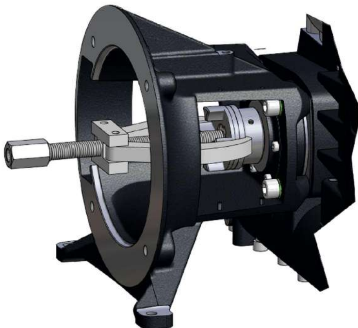
Figure 8-4 – COUPLING REMOVAL TOOL – VS40 MODEL SHOWN
