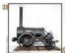
1829 Robert Stephenson built the Rocket. It was a steam engine. It was built for a contest to show off the best engine. It reached 30 miles per hour. Many steam engines since have been modeled on the Rocket.
