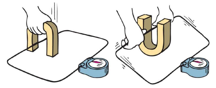
Voltage is induced in the wire loop whether the magnetic field moves past the wire or the wire moves through the magnetic field.
