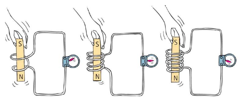
When a magnet is plunged into a coil with twice as many loops as another, twice as much voltage is induced. If the magnet is plunged into a coil with 3 times as many loops, 3 times as much voltage is induced.
