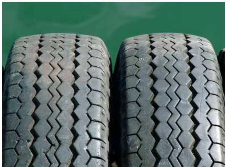
Figure 2.1.8. Two tires of the same make and model. The model is a form of class information while the damage seen along the right rim of the right tire is a form of individual evidence ( www.ehow.com/how_7536688_identify-tire-tracks.html ).
