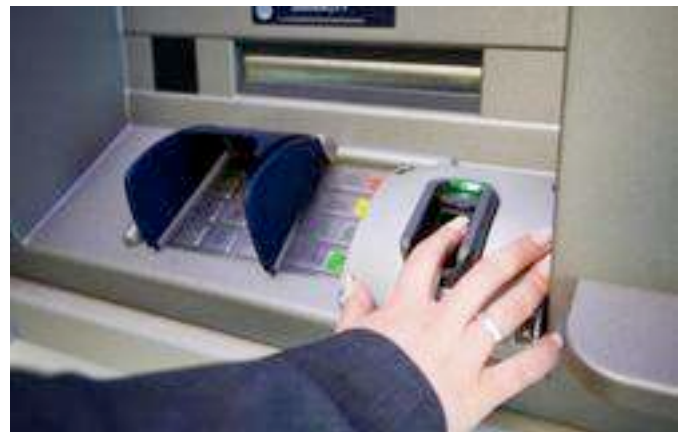
Figure 2.1.6. Personal identification authentication on an automated bank teller device using fingerprint recognition to verify a person’s identity by matching the scanned fingerprint at the beginning of the transaction with a reference previously taken from the person and stored in a databank ( www.homelandsecuritynewswire.com/topics/authentication-biometrics?page=2 ).
