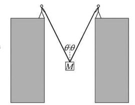
**PART B:** Derive an expression for the magnitude of the tension  $F_T$  in the two ropes in terms of M,  $\theta$ , and fundamental constants.
