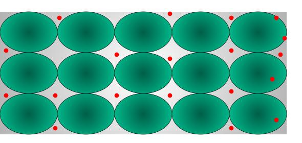
When the metal is heated, this 'sea of electrons' gain kinetic energy and transfer it throughout the metal.
