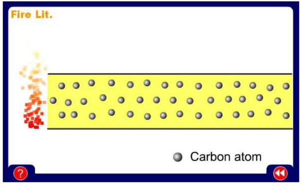
As you heat the metal, the particles vibrate, these vibrations make the adjacent particles vibrate, and so on and so on, the vibrations are passed along the metal and so is the heat. We call this?
