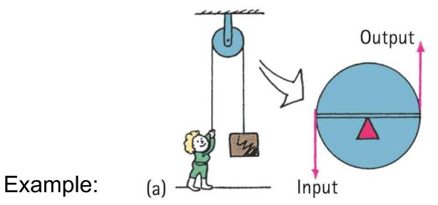
This pulley arrangement can allow a load to be lifted with half the input force.
