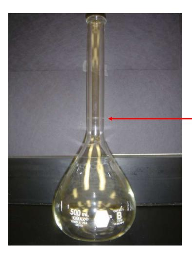
A volumetric flask is used to measure an exact quantity of a liquid. Notice the single white line on the column of the container!
