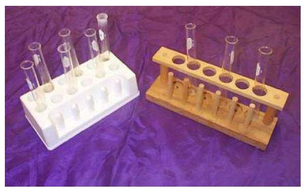
Test tube racks are for holding and organizing test tubes on the laboratory counter. Plastic racks may melt when in contact with very hot tubes.
