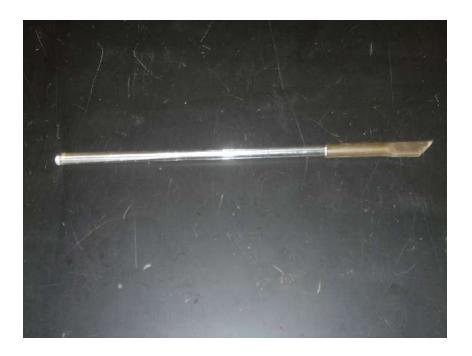
A glass stir rod is used to manually stir solutions. It can also be used to transfer a single drop of solution.
