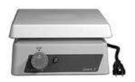
A hot plate is used as an alternate heat source from the bunsen burner.
