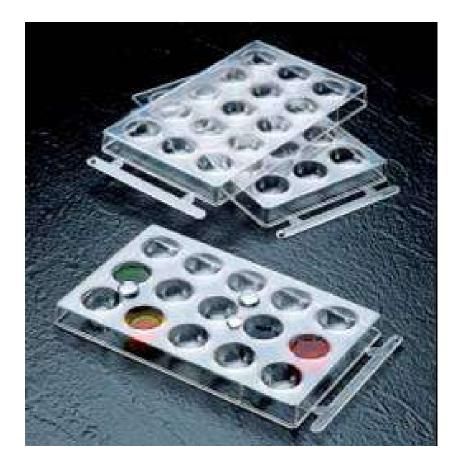
Spot plates are used to perform many small scale reactions in one location.
