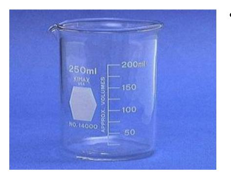
Beakers hold solids or liquids that will not release gases when reacted or are unlikely to splatter if stirred or heated.
