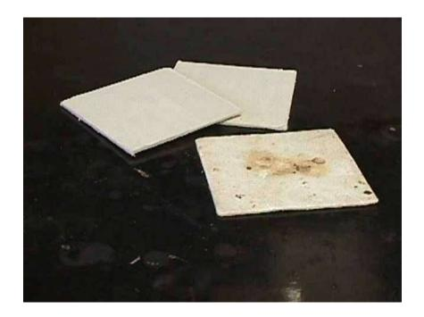
A 4" x 4" square of ceramic fiber provides a surface for hot beakers so that the beaker does not come into contact with a cold countertop and shatter.
