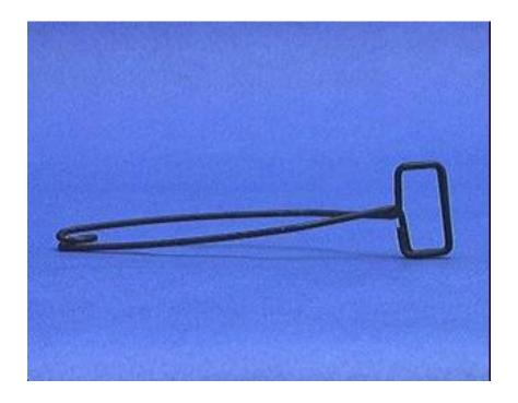
A test tube holder is useful for holding a test tube which is too hot to handle.
