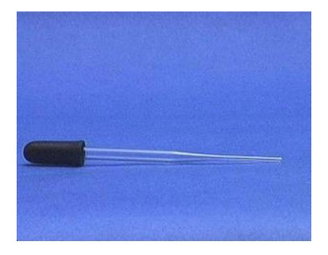
A medicine dropper is used to transfer a small volume of liquid (less than 1 mL).
