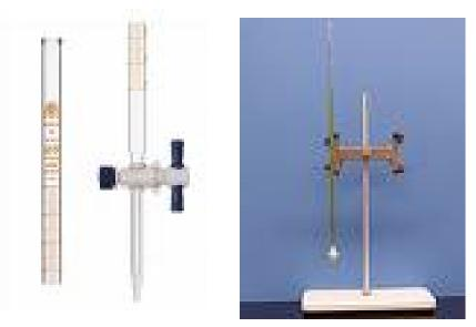
Double buret clamps are used to secure burets for reactions.
