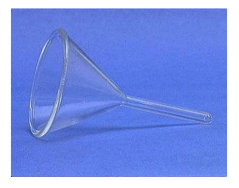
A funnel is used to aid in the transfer of liquid from one vessel to another.
