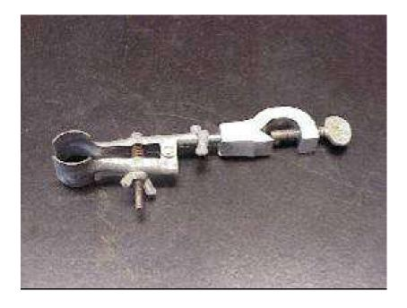
Utility clamps are used to secure test tubes, distillation columns, and burets to ringstands.
