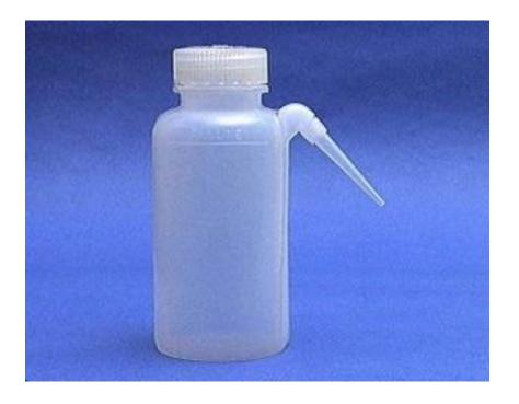
A wash bottle has a spout that delivers a wash solution to a specific area. It is also good for rinsing solids from beakers. Distilled water is the only liquid that should be used in a wash bottle.
