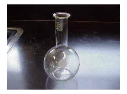
Used sparingly in general chemistry – it is used for the mixing of chemicals. The narrow neck prevents splash exposure.
