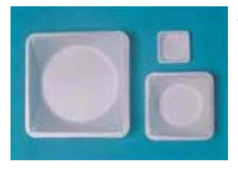
Weighing boats are used to weigh solid that will be transferred to another vessel. No material should ever be placed "naked" on a scale or balance.
