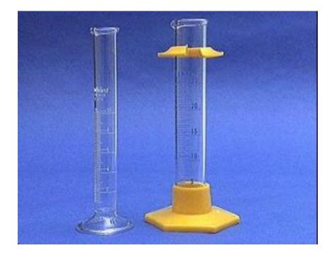
A graduated cylinder is used to measure volume of liquids.
