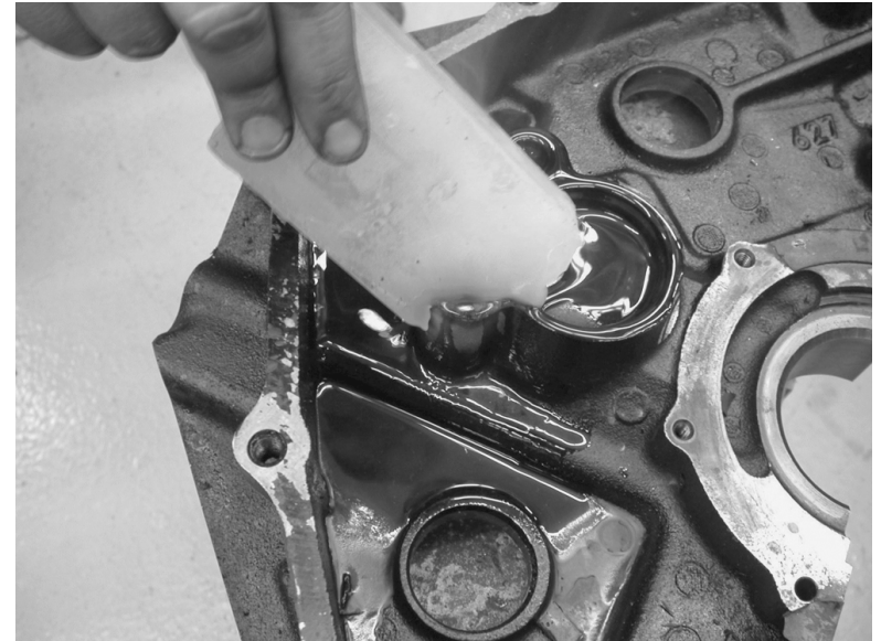
FIGURE 4-40 Removing plugs or bolts is easier if the plug is first heated to cherry red color, using a torch, and then applying wax. During cooling, the wax flows in between the threads, making it easier to remove.
