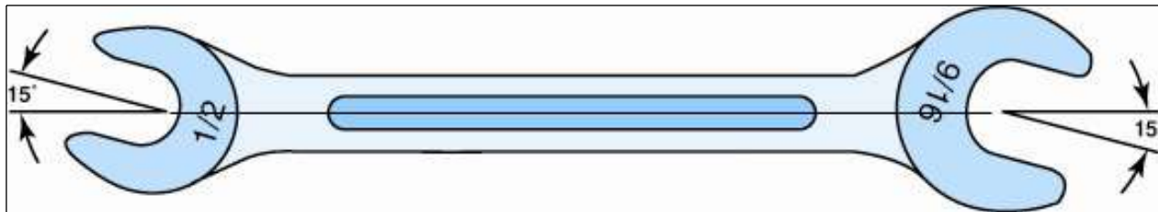
FIGURE 4-2 A typical open-end wrench. The size is different on each end. Notice that the head is angled 15 degrees at each end.
