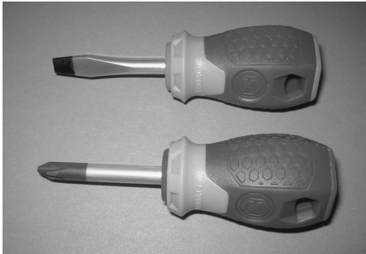
FIGURE 4-18 Two stubby screwdrivers that are used to access screws that have limited space above. A straight blade is on top and a #2 Phillips screwdriver is on the bottom.
