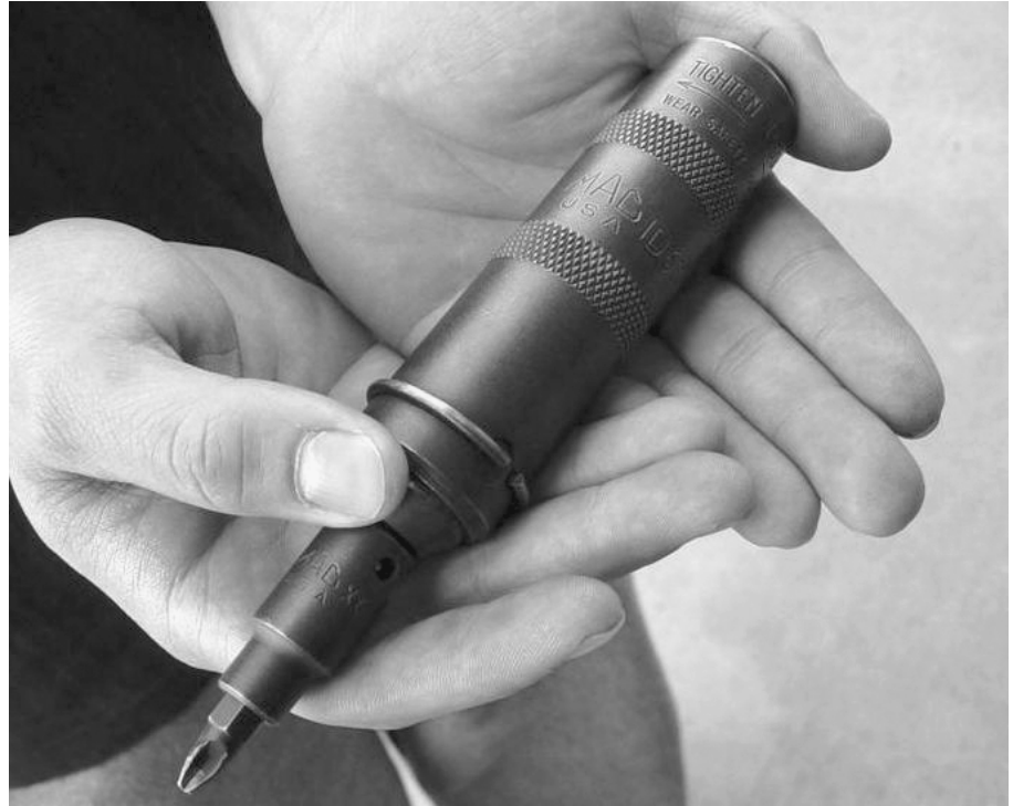
FIGURE 4-20 An impact screwdriver used to remove slotted or Phillips head fasteners that cannot be broken loose using a standard screwdriver.
