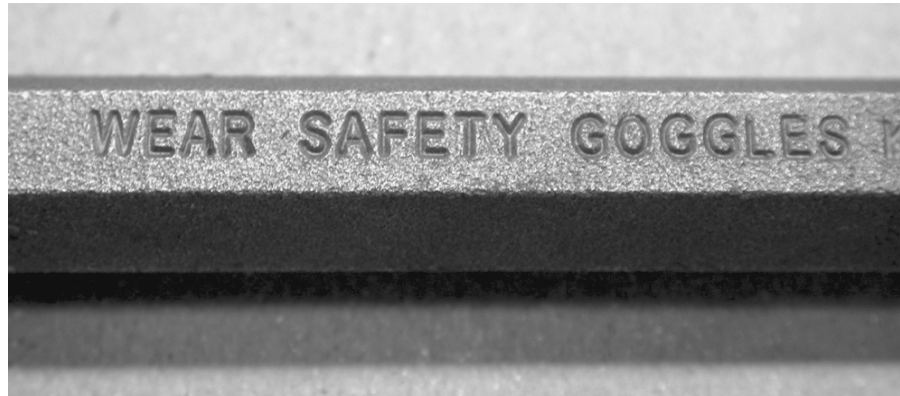
FIGURE 4-35 Warning stamped in the side of a punch warning that goggles should be worn when using this tool. Always follow safety warnings.
