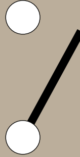
SWITCH OPEN (OFF)
