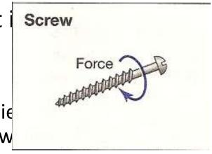
bThe amount of work for a screw depends on the number of thread, which is actually the length of the inclined plane
