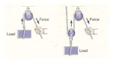
bA double pulley makes work easier not only by changing the direction of the force, but also by multiplying the effort
