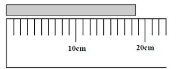
This ruler is not as precise (due to having less markings). The length looks to be between the 10 and 20cm. So we can estimate the last digit to be 12cm or 13cm. This will give the measurement 2 sig figs. \*\*The last number is the estimated digit
