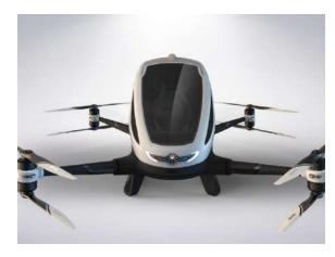
press a launch button. From there, the 440-pound drone will lift off and begin flying. What's more, EHang says that its drone will be an extremely safe ride. Made from a composite material, carbon fiber, and epoxy, the flying machine is programed with multiple emergency plans that, in theory, have the ability to safely fly its passenger to the nearest landing location.
