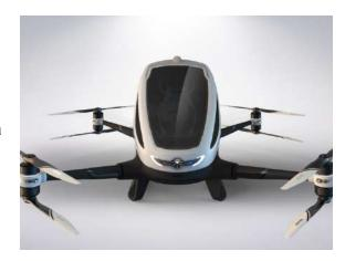
press a launch button. From there, the 440-pound drone will lift off and begin flying. What's more, EHang says that its drone will be an extremely safe ride. Made from a composite material, carbon fiber, and epoxy, the flying machine is programed with multiple emergency plans that, in theory, have the ability to safely fly its passenger to the nearest landing location.
