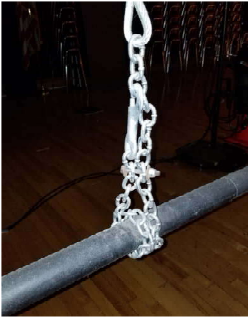
3 EXAMPLES: IMPROPER TRIM CHAINS
