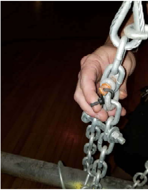
3 EXAMPLES: IMPROPER TRIM CHAINS
