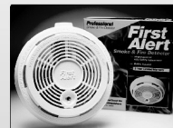
A household smoke detector uses radioactive americium-241. This alpha emitter has a half-life of 432 years. In a smoke detector the emission ionizes smoke particles to activate the alarm. (Charles D. Winters)
