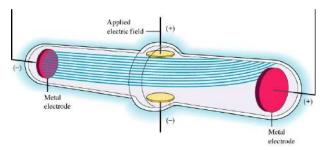
o He then measured the deflection of beams of e to determine the charge-to-mass ratio
