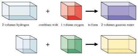
1 volume hydrogen combines with 1 volume chlorine to form 2 volumes hydrogen chloride
