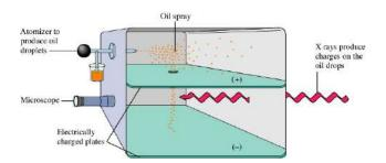
1909 Robert Millikan, American—University of Chicago, sprayed charged oil drops into a chamber. Next, he halted their fall due to gravity by adjusting the voltage across 2 charged plates. Now the voltage needed to halt the fall and the mass of the oil drop can be used to calculate the charge on the oil drop which is a whole number multiple of the electron charge. Mass of e<sup>-</sup> = 9.11 × 10<sup>-31</sup> kg.
