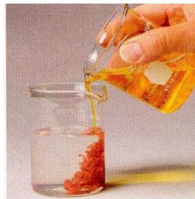
A potassium chromate solution being added to aqueous silver nitrate, forming silver chromate.
