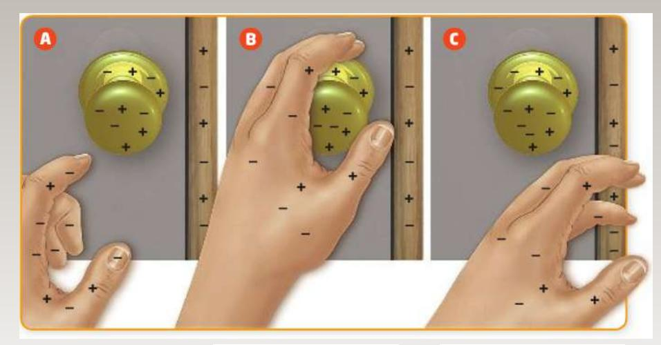
A The hand has a negative charge (a surplus of electrons). **B** If the hand touches the metal doorknob, there is a rapid transfer of electrons, and a shock is felt.
