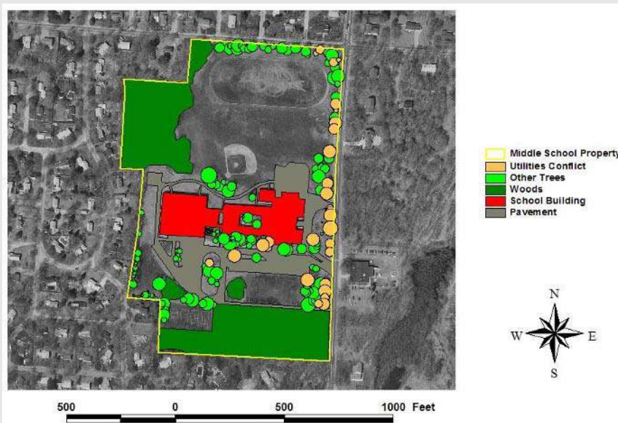
FIGURE 8.5 Trees conflicting with utility lines.
