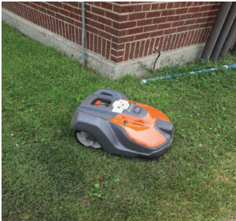
Part of the energy-friendly landscaping services are 29 robotic lawnmowers that whirl around the 65-acre campus. Like an indoor Roomba, each robot mows a declared area outside and when done, returns to its charging base. They are satellite-driven and can be programmed to cover any area that needs mowing. The students, of course, are fond of the robots, have given them names, and, on occasion, decorated them with googly eyes.
