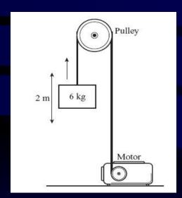
The motor is lifting the 6 kg box at a constant velocity. How much work is done on the box to lift it 2 m? (Assume no resistance from the pulley.)
