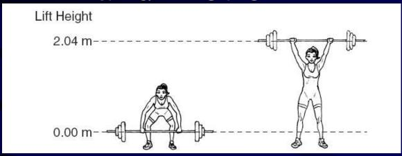
The weight lifter used a force of 980 N to raise the barbell over her head in 5.21 seconds.
