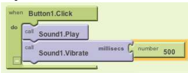
Figure 1-14. Plug the 500 into the milliseconds slot.
