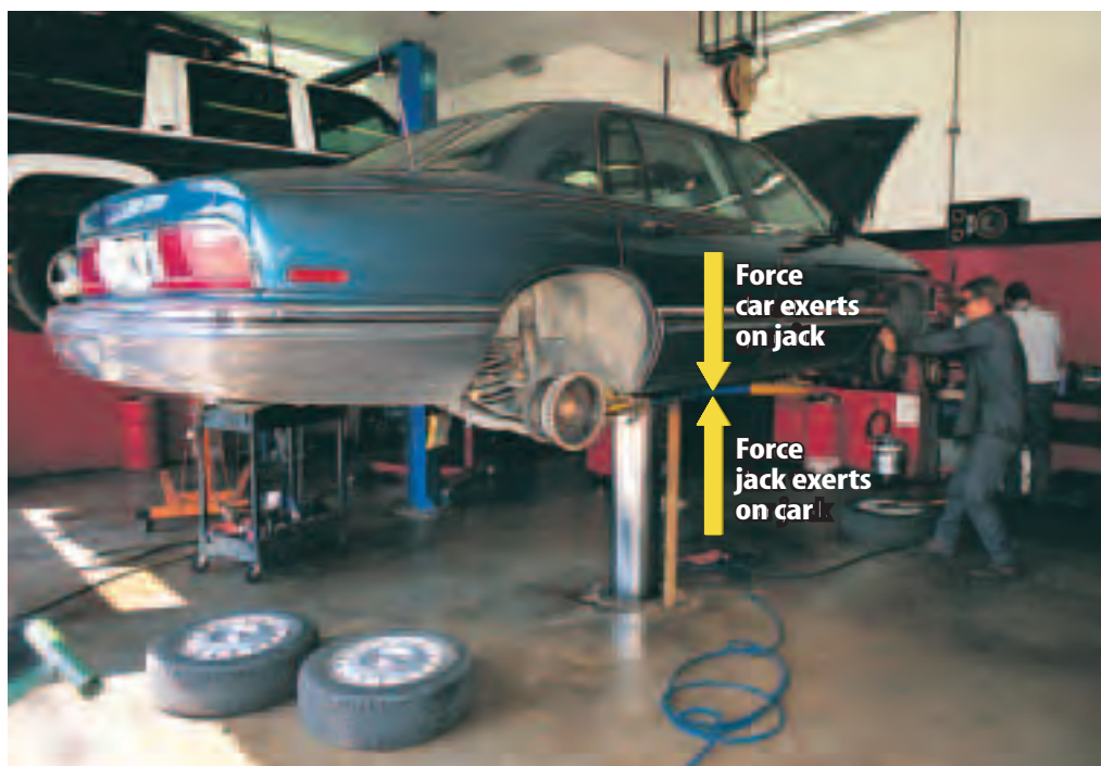
Figure 13 The car jack is pushing up on the car with the same amount of force with which the car is pushing down on the jack. Identify the other force acting on the car.
