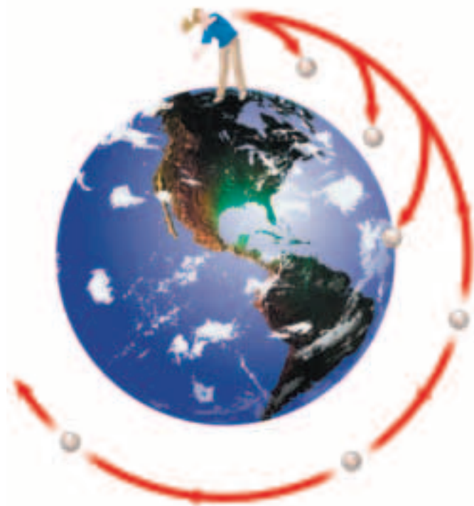
Figure 11 The faster a ball is thrown, the farther it travels before gravity pulls it to Earth. If the ball is traveling fast enough, Earth's surface curves away from it as fast as it falls downward. Then the ball never hits the ground.
