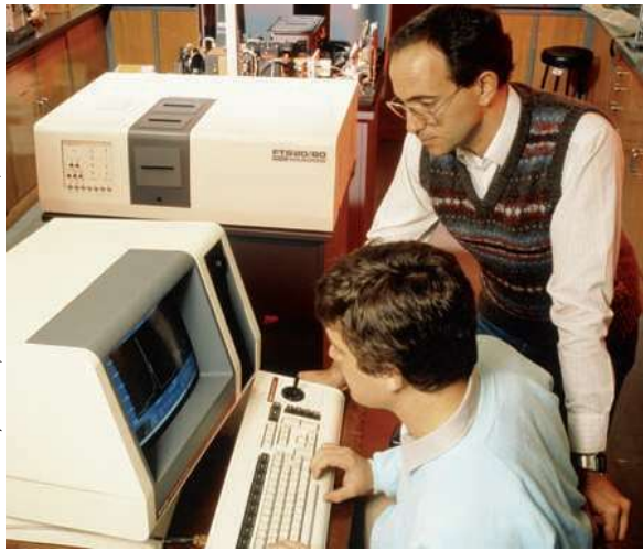
Figure 4-3. An infrared spectrometer is used to identify unknown fibers.
