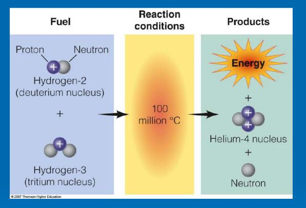
Nuclear fusion: two isotopes of light elements are forced together at extremely high temperatures until they fuse to form a heavier nucleus.
